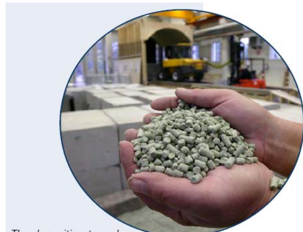
The deposition tunnels will be filled with blocks and pellets made of bentonite clay.
